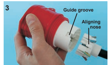
Fit distributor ring onto front part. Important: Aligning nose provides for correct position when inserted in guide groove.
