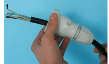
Remove approx. 35 - 40 mm of the sheathing from the cable (with 6 mm 2 45 mm) and feed it through the back part from behind. Cut off the non-conductive core.
